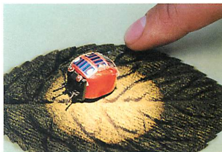
Fig. 2 Photon energy supply to the insect-shaped actuator
