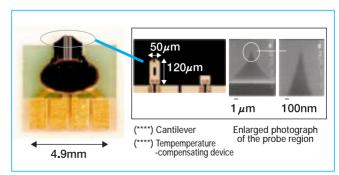
Fig. 1 Photomicrograph of an AFM cantilever
