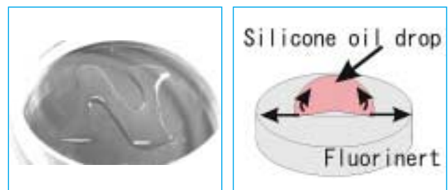
Fig. 1 The path of flow is formed by wettability distribution
