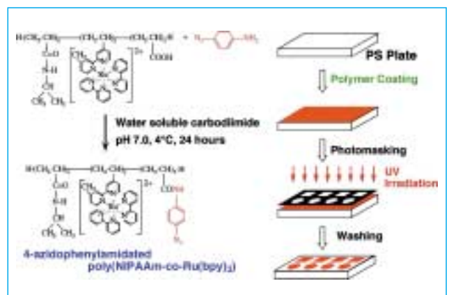
Fig. 1 Gel micromachining through photolithography
