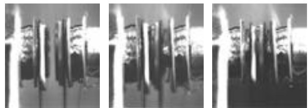
(a) Separated state (b) Excited state (c) Connected state Fig. 2 Movement of microconnector
