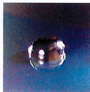
Fig. 3 Water contact angle on deposited Teflon-like film
