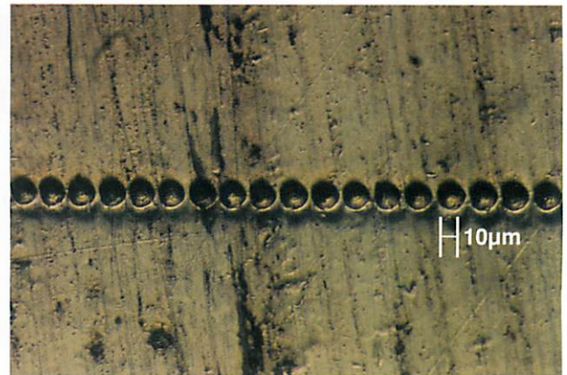
Fig. 4 Surface of material after dynamic indentation
