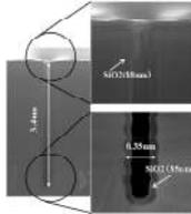
Supercritical-fluid conformal deposition
