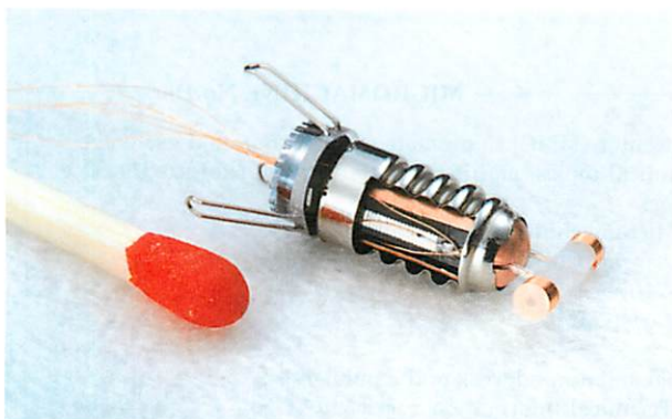
Fig.2 Micro Inspection Machine by Denso Corp.
