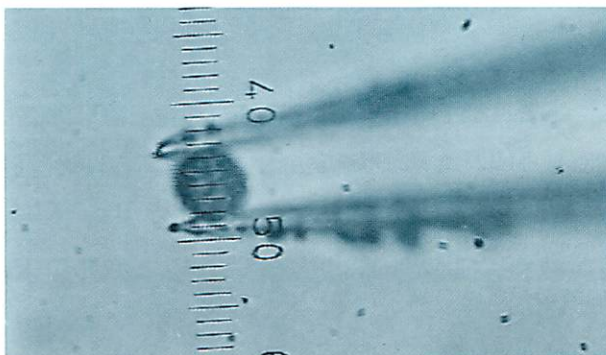
Fig. 5 Micro Manipulation of Latex Particles (5 \mu\text{m} dia.) (Mechanical Engineering Laboratory, AIST, MITI.)
