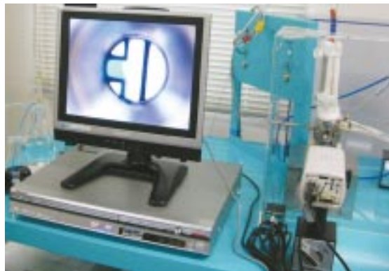
Cell system for visual observation of supercritical mixtures (jointly developed with Takafumi Aizawa, senior research scientist at AIST Research Center for Compact Chemical System)
