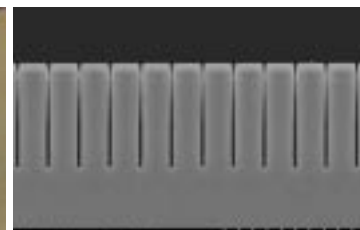
Figure 2. High aspect etching using the NLD-Si method
