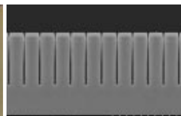
Figure 2. High aspect etching using the NLD-Si method
