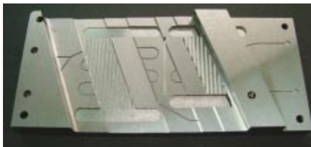
Fig. 3 Layered heat exchanger cut to show the internal structure (manufactured by Yachida)
