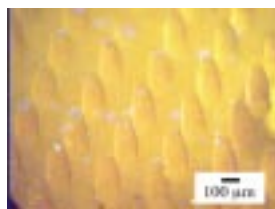
Fig. 2 Gel array created through micromachining (artificial cilia)
