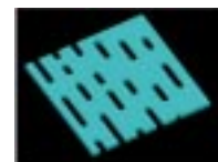
Pit pattern in an optical disc formed by direct electron beam writing
