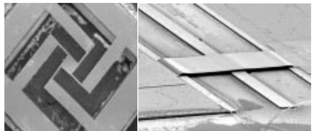
An optical scanner using ferroelectric material (left) and an RF switch driven by a low voltage
