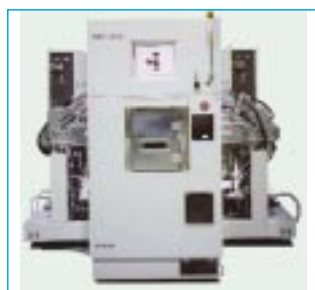
SME-200 PVD device for forming high-dielectric films and MEMS electrodes
