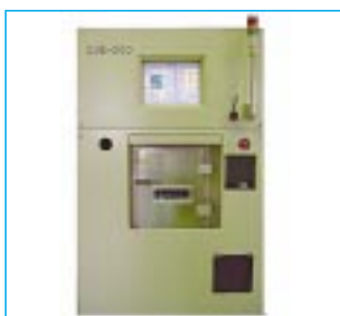
CME-200 PE-CVD device for forming SiO 2 and SiN x films
