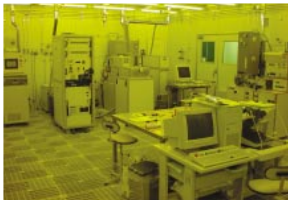
Fig. 1 Class 1000 Clean Room (70m 2 )
