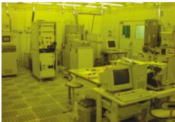
Fig. 1 Class 1000 Clean Room (70m 2 )
