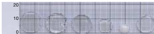
Fig. 1 Dependence of the volume of a cross-linked MPC polymer gel on alcohol composition Ethanol composition (from left): 0, 20, 40, 60, 80, and 100%
