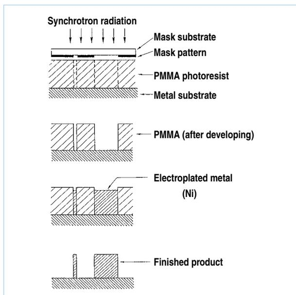
Fig. 3 Cross-sectional view of the LIGA process.
