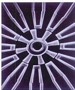
Fig. 1 Electrostatically driven micromotor made of polycrystalline silicon film (Courtesy of Prof. M. Mehregany, Case Western Reserve Univ. USA)
