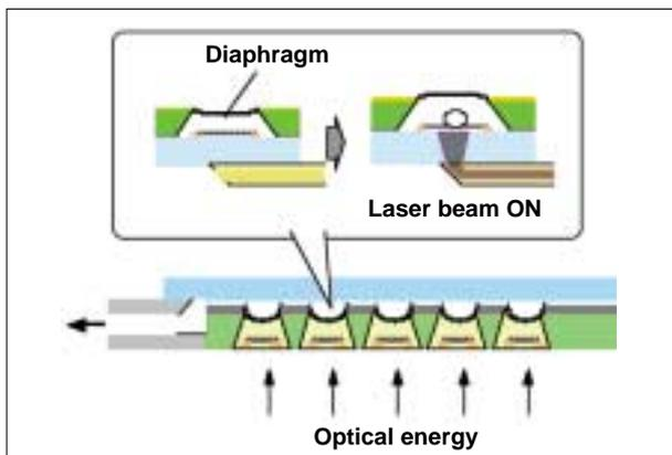
Fig. 1 Principle of Peristaltic Micropump
