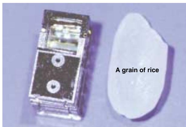
Fig. 1 Micro Optical Scanning Sensor
