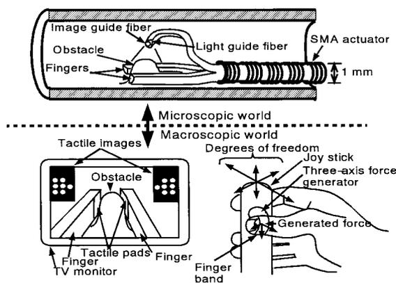
Fig. 1 Tactile Microsensor/Tactile Information Display System
