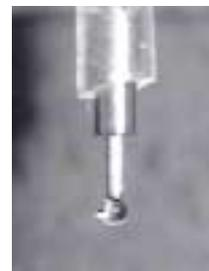
Fig. 3 How Trace Amounts of Adhesive are Discharged
