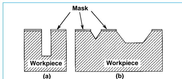
Fig. 2 Cross Section Resulting from Anisotropic Etching
