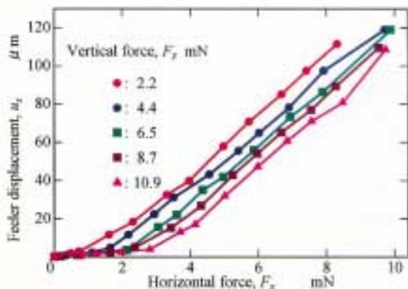
**Fig. 5 Horizontal Force Detection Characteristics**
