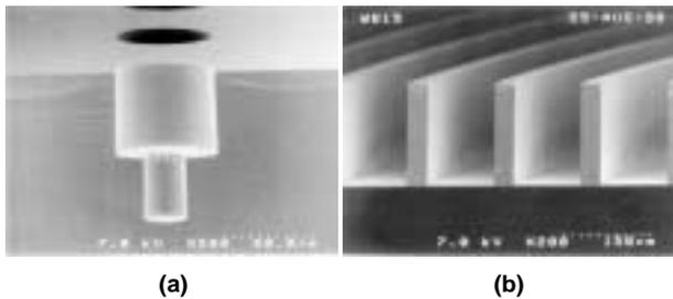
**Fig. 3 Examples of Machined Ink-Jet Printer Heads**
