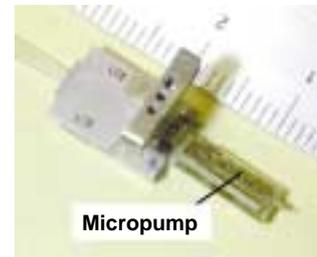
Fig. 2 Light-driven Coating Device
