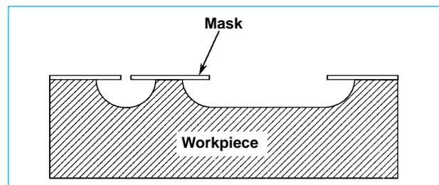
Fig. 1 Cross Section Resulting from Isotropic Etching
