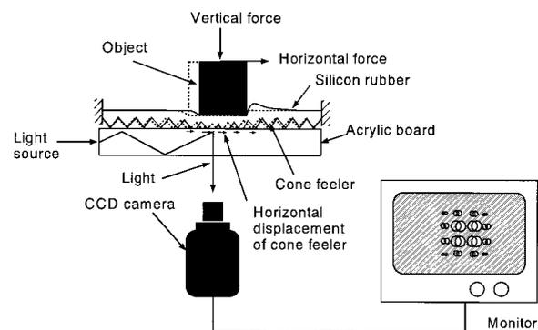
Fig. 2 Principle of Tactile Microsensor
