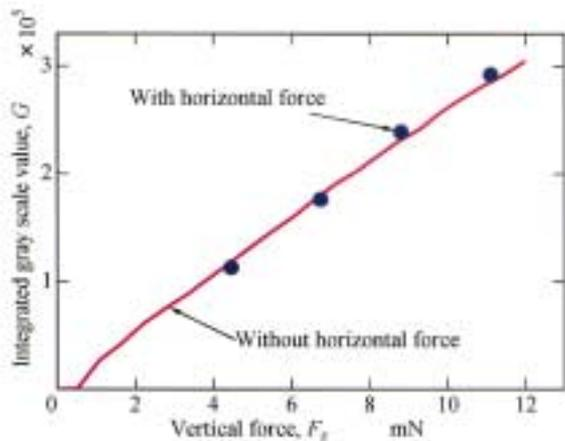
**Fig. 4 Vertical Force Detection Characteristics**
