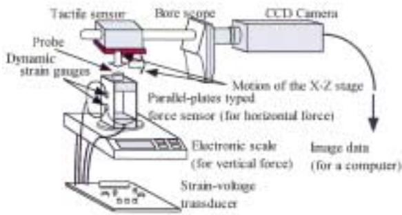
**Fig. 3 Prototype of Tactile Microsensor System**
