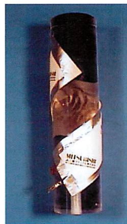
Fig. 2 Flexible shaped battery folded round the tube
